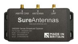
The SM2000 range of Diplexers are designed to provide an improvement of VSWR between a multiple transmitters and one aerial. In order to maintain this enhanced performance it is necessary to minimize insertion losses through the system. The SM2000 is designed with a very low insertion loss factor of less than -0.3 dB at VHF, and Port to Port Isolation of better than -40dB. This, together with its capability to improve
